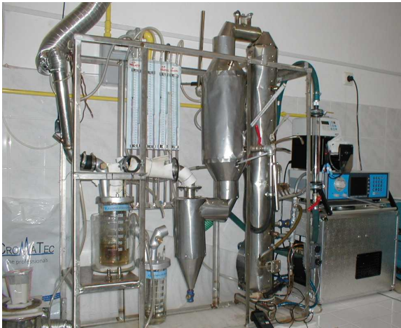
Figure 4: Experimental Lab scale facility for testing the Hg retention (photo and schematics):
