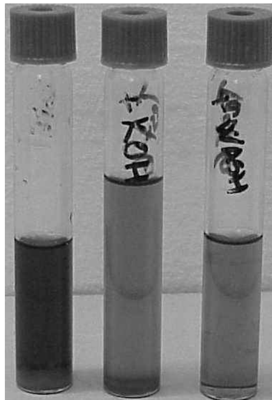
Figure 4: Probe No. 6 after second step(left), after third step with KOH (middle) and after washing (right)
